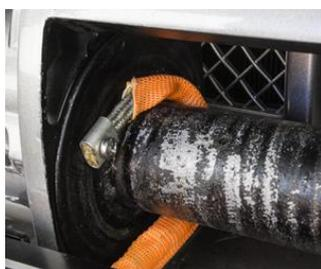
You can see in this picture how the rope is spooled on underneath the drum and attaches using the drum link and button head screw.
