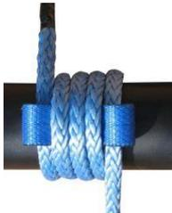
**Step 3:** Loop the winch rope around the drum once or twice more and then attach the terminal end of the winch rope to the winch drum. Pull the winch rope arranging the loops side-by-side at the attachment side of the winch drum. Now you are ready to spool in the rest of the winch rope under load.
