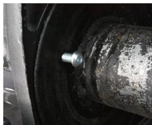
There are two main ways that winch lines attach to the drum, either with a screw on the side of the drum or through a hole in the centre of the drum itself. Here you can see the button head screw that holds a terminal onto the winch. If you have this setup then you just need to simply bolt the connector link on the end of the winch line to your winch with the provided screw.
