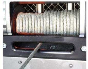
As stated before, it is best to have two people to install a winch line. It can be difficult to simultaneously guide the winch line in correctly and handle the winch controller.
