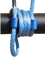
**Step 2:** Pull about 800mm of the winch rope through and wrap 4 to 5 times over the winch rope retainer. Make sure to wrap in the correct direction (winch line typically comes off the lower side of the winch drum). Then put the winch rope through the other loop in the winch rope retainer and pull it through.
