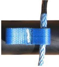
**Step 1:** Insert the terminal end of the winch rope through the aluminium Hawse fairlead on the front of the winch and through one loop of the winch rope retainer.
